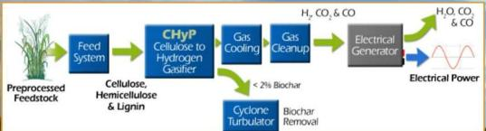
Pyrolysis systems generate hydrogen-rich gas streams from biomass to power and heat generation. (Cellulose to Hydrogen Power system, or CHyP system)
